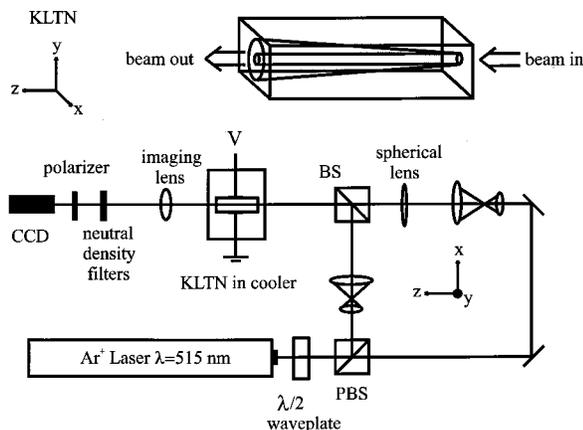
FIG. 2. Experimental setup and crystalline configuration.
