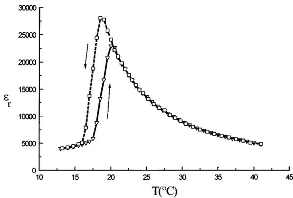
FIG. 1. Measured values of  $\epsilon_r$  as a function of temperature  $T$ . The two curves represent values measured for decreasing (squares) and increasing (triangles) temperatures.
