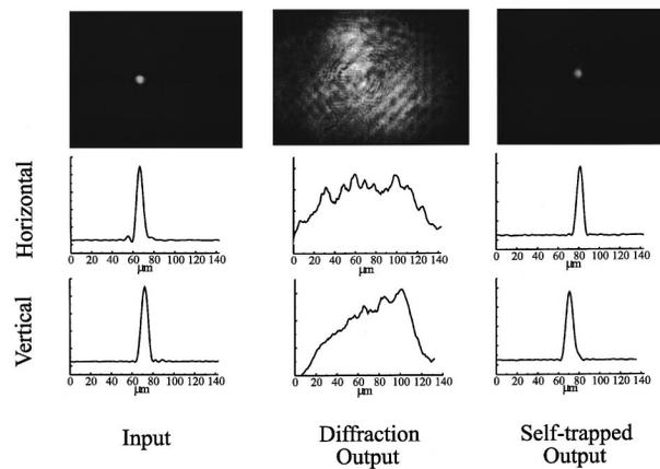
FIG. 3. Photographs and profiles of the beam at the input and output faces of the crystal.
